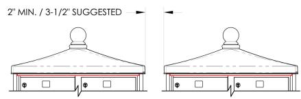
IMPORTANT CLEARANCE SPEC SEE MULTI UNIT PAD SPECIFICATION FOR BOLT PATTERN AND SPACING
