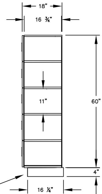
(BASES ARE MADE OF INDUSTRIAL GRADE PARTICLEBOARD AND ARE COVERED IN A DURABLE BLACK LAMINATE. PLEASE SET BASE TO ALLOW 5/8" BETWEEN THE BACK OF THE LOCKER AND THE WALL FOR AIR VENTILATION.)
